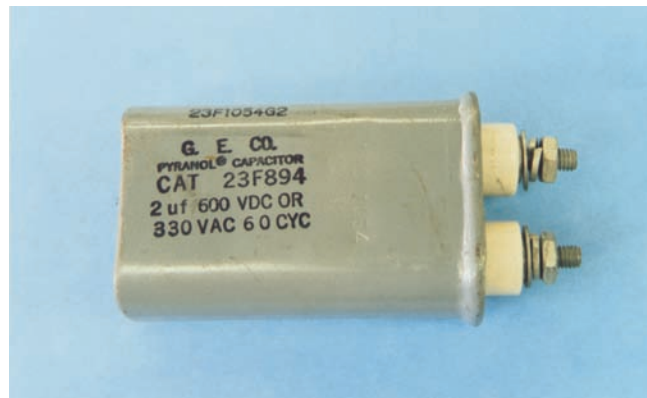
FIGURE 20-18 Oil-filled paper capacitor.
