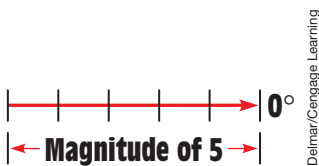
FIGURE 15–11 A vector with a magnitude of 5 and an angle of 0^\circ .
