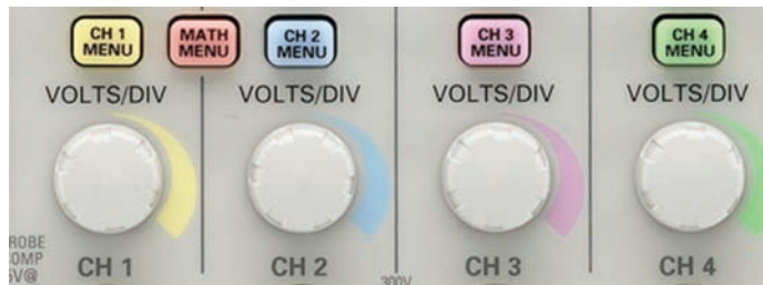
FIGURE 10-48 Voltage control knobs of a four channel digital oscilloscope.
