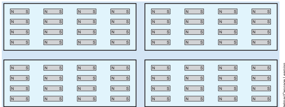
FIGURE 4-7 When a magnet is cut apart, each piece becomes a separate magnet.
