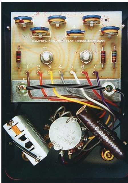
FIGURE 10-23 DC ammeter with an Ayrton shunt.
