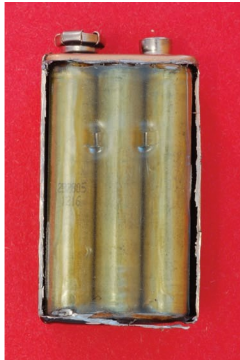
FIGURE 13-12 Internal makeup of a 9-V battery.
