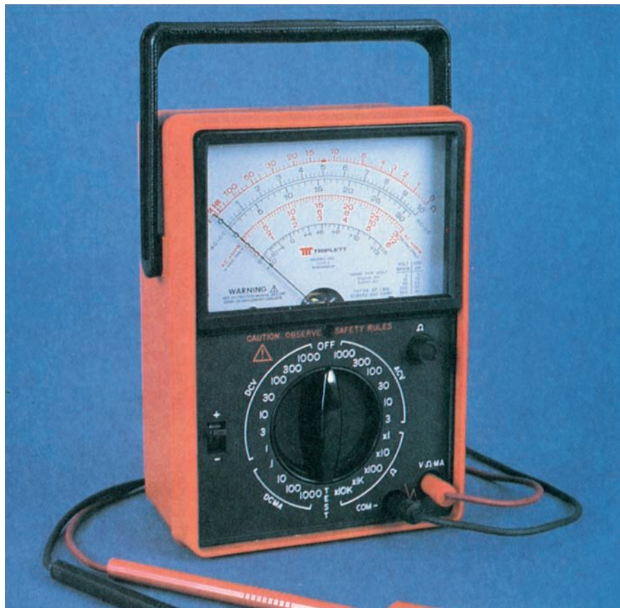
FIGURE 10-6 Volt-ohm-milliammeter with multirange selection.
